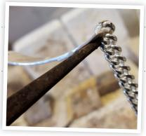
tightly. Hold the link at the bottom with your soldering pliers, so the cut is raised above the silver rectangle. This is fiddly, but worth it as you will not end up soldering the chain to the rest of the silver! Apply a small amount of solder paste to the cut, and solder closed.
