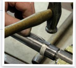
the lead onto the soldered seam. This will gently lay the seam flush on the inside without distorting the main body. Finally using a fine file clean any excess solder and material from the outside edge.
