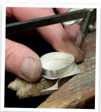
will help to protect the polished surfaces from fire stain. Allow the meths to dry or gently burn off. Then apply a small piece of hard solder to the outside base of the main body and coax it around using the soldering probe. This will enable the use of less solder. Allow to cool and place in a pickle to clean. Once clean and dry, cut the excess material away using a piercing saw.
