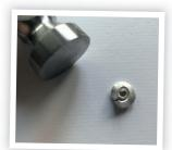
Once you are happy with the shape of your rose, give it a gently whack to make sure that the edges on the reverse are flush. This is important so that the solder with flow and attach the rose to the cuff.
