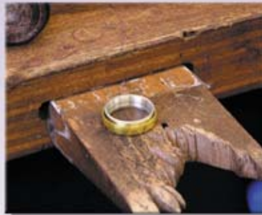
2) The concave ring is then stretched into place behind the inserted ring.
